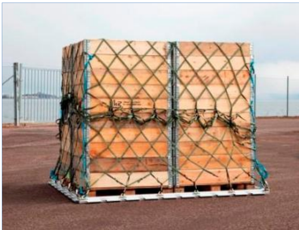
Figure 5.1: Single base plate of the conventional aluminum sheet military aircraft pallet.
