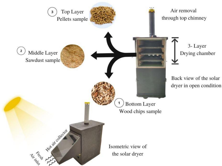
Figure 8. Experimental setup of the solar dryer for the investigations.
