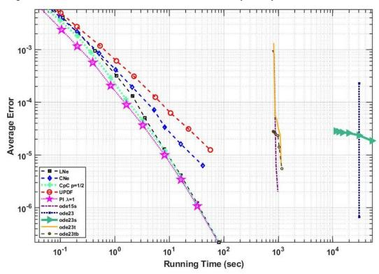
**Figure 4.2.** (average) errors as a function of the running time for the first (moderately stiff) system, in the case of the algorithms coded by us as well as of the MATLAB routines.
