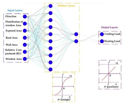
Figure 7.1. A schematic diagram of the ANN and its relation to the input and output parameters.
