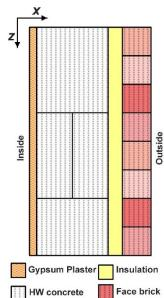
Figure 7.7. Cross section of a four-layer wall.
