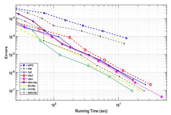
**Figure 3.4.** The  $L_{\infty}$  errors as a function of the running times for the (very Stiff) system, in the case of the UPFD, CNe, CpC, LNe2, LNe3, the OEH-CNe, the SH-CNe, the LH-CNe and the ASH-CNe methods.
