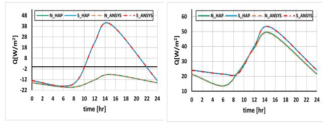
**Figure 8.8.** Comparison for the optimal roof, based on HAP and ANSYS (N-north side roof, and S-south side roof) result. Left side: winter in Hungary, Miskolc. Right-side: summer in Baghdad, Iraq.
