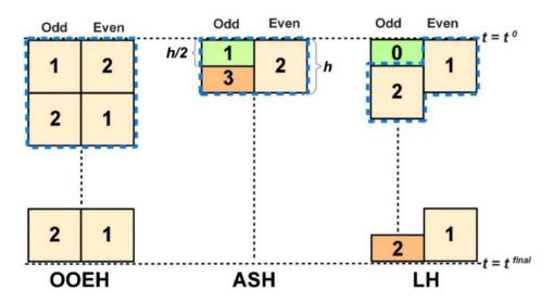
**Figure 2.2.** Hopscotch-type space-time structures. The time elapses from the top  $(t = t^0)$  to the bottom
