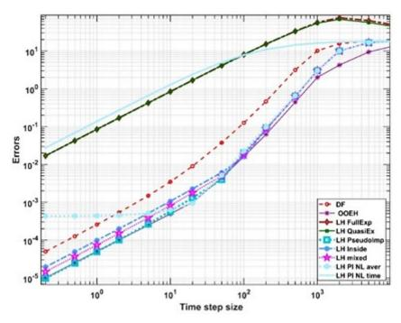
**Figure 5.3.** The maximum errors as a function of the time step size for the nine examined methods in the case of a surface area (Section 5.2.4 Part II). For the radiation term.
