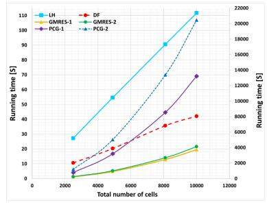
**Figure 6.7.** The running time with total number of cells for  $\Delta t = 1$  s. The left-hand side vertical axis refers to the LH and DF methods, while it is on the right-hand side axis for the implicit methods.
