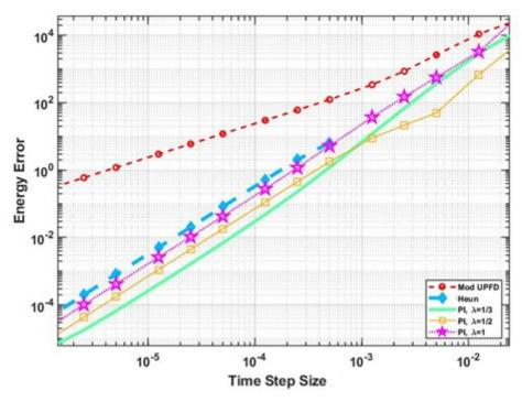
**Figure 4.3.** Energy errors as a function of the time step size for the second (very stiff) system, in the case of the UPFD Algorithm 2, the Heun method and the new PI algorithms.
