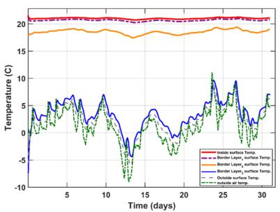
**Figure 7.8.** The temperature distribution in °C as a function of time in days for the four-layer wall facing North. Border layer means the boundary between two different materials (Border 1 between gypsum plaster and heavy-weight concrete, Border 2 between HWC and insulation, and Border 3 between insulation and face brick.).
