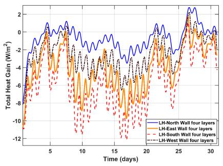
Figure 7.11. Total heat gain distribution in W/m<sup>2</sup> as a function of time in days for the wall simulation facing North, East, South, and West.
