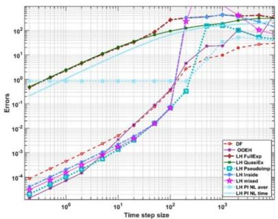
**Figure 5.6.** The maximum errors vs. the time step size h for the non-equidistant mesh (Section 5.2.5 Part II) in the case of convection and radiation boundary conditions.
