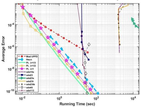
**Figure 4.4.** (average) errors as a function of the running time for the second (very stiff) system, in the case of the new algorithms and some other methods.
