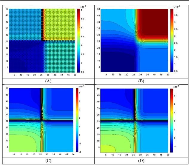
**Figure 6.8.** The error of temperature distribution contour in Kelvin units (A) LH, (B) DF, (C) GMRES and (D) PCG methods.
