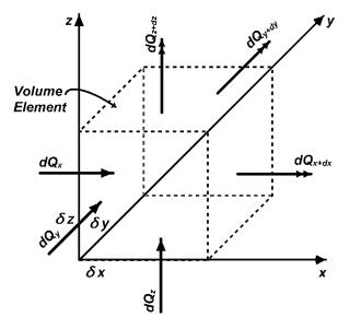
Figure 1.2. Which is used for deriving heat conduction in Cartesian coordinates, the volume is defined by  $\delta x$ ,  $\delta y$ , and  $\delta z$ .
