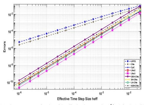
**Figure 3.1.** The  $L_{\infty}$  errors as a function of the effective time step size ( $\Delta t_{EFF}$ ) for the (Mildly Stiff) system, in the case of the UPFD, CNe, CpC, LNe2, LNe3, the OEH-CNe, the SH-CNe, the LH-CNe and the ASH-CNe methods.
