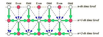
Figure 2.3. The stencil of the original odd-even hopscotch algorithm. Thin blue arrows and thick green arrows indicate operations at the first stage and second stage, respectively.
