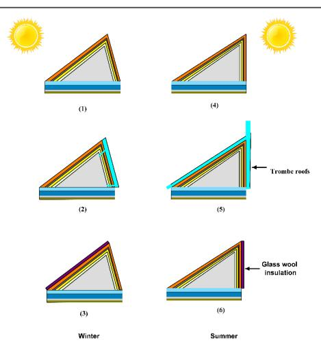
**Figure 8.6.** Illustration of the cases I simulated, including optimal roof, roof with Trombe, and glass wool insulation on one side of roof. The roofs on left side winter season and right side summer season.
