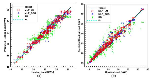
Figure 7.4. The result of R<sup>2</sup> values for the data predicted by three neural networks: MLP\_LM, MLP\_SCG, and RB (a) for the heating load and (b) for the cooling load.
