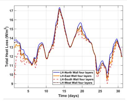
Figure 7.9. Total heat loss distribution in W/m<sup>2</sup> as a function of time in days for the wall simulation facing North, East, South, and West.
