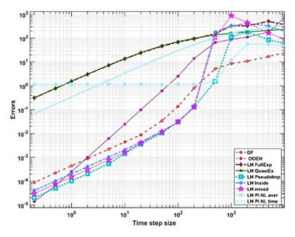
**Figure 5.5.** The maximum errors as a function of h for the equidistant mesh (Section 5.2.5 Part I) in the case of convection and radiation boundary conditions.
