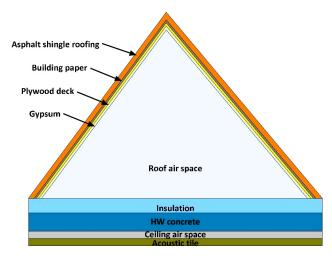
Figure 8.1. The materials used in the roof and ceiling.
