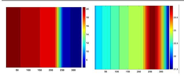
**Figure 7.12.** Contour of the temperature distribution in °C on the South-facing side of the building for two different seasons: winter (left) and summer (right).
