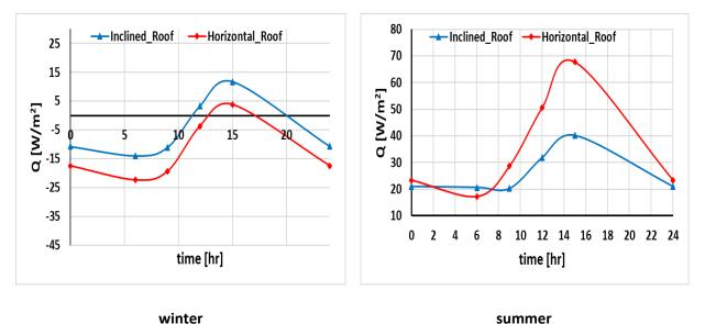
Figure 8.5. Roof heat loss and gain with time on left side winter season and right-side summer season. 8.2.2. ANSYS simulation
