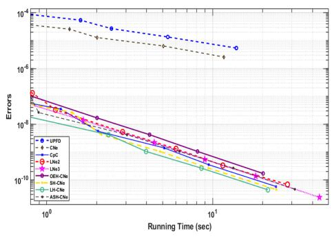
Figure 3.2. The  $L_{\infty}$  errors as a function of the running times for the (mildly stiff) system, in the case of the UPFD, CNe, CpC, LNe2, LNe3, the OEH-CNe, the SH-CNe, the LH-CNe and the ASH-CNe methods.
