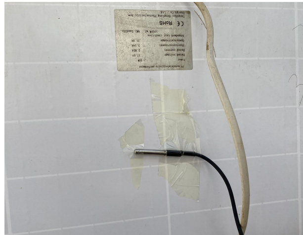
Figure 3.27: Placement of DS18B20 temperature sensors at the rear center of PV panels.
