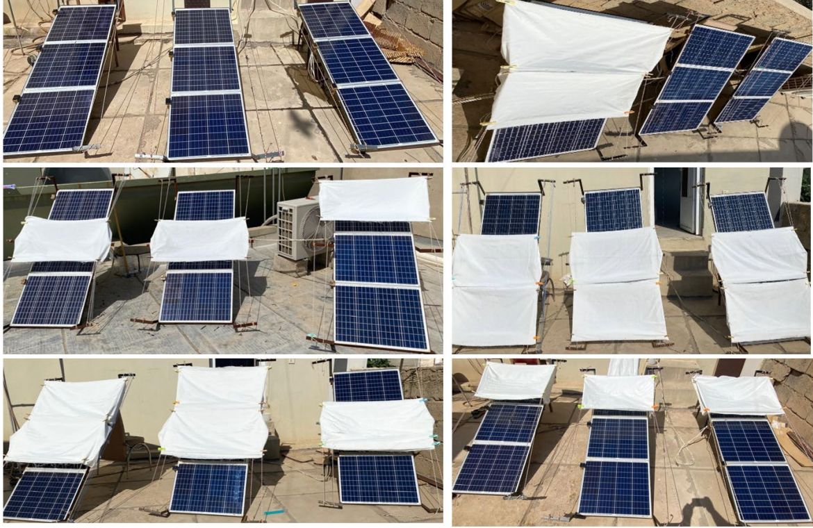
Figure 7.1: Different stages of shading applied using fabric layers.
