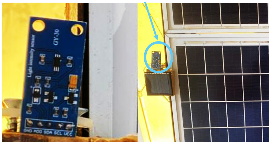
Figure 3.26: The light intensity sensor (BH1750) positioned adjacent to the PV panel.
