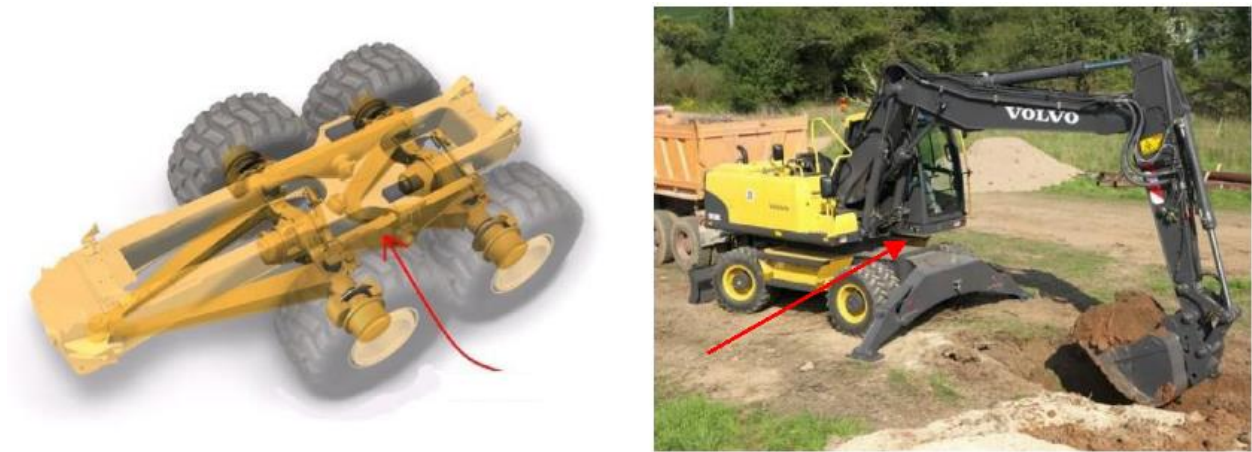
Fig. 2.14. Boggi beam (left) and excavator arm (right) [33].
