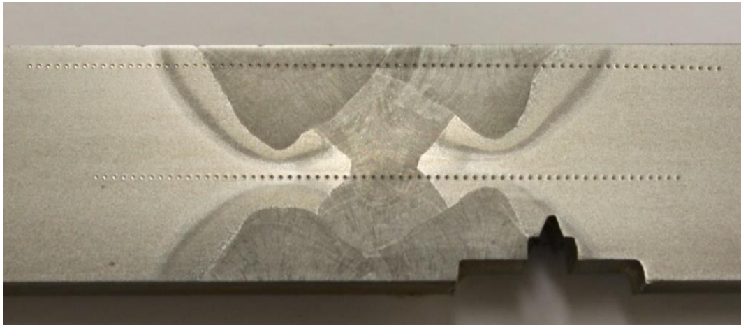
Fig. 5.6. Macro-structure of the M/OM welded joint with a notch location and hardness indentations.
