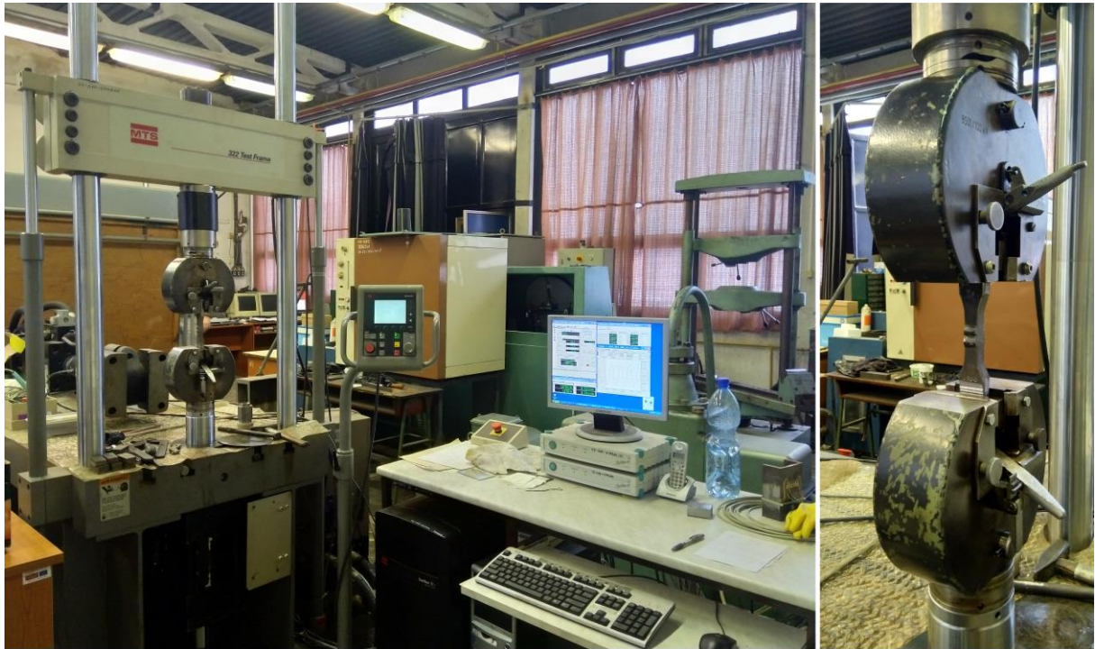
Fig. 6.1. MTS type electro-hydraulic testing system equipped for the HCF investigation of butt welded joint specimen.
