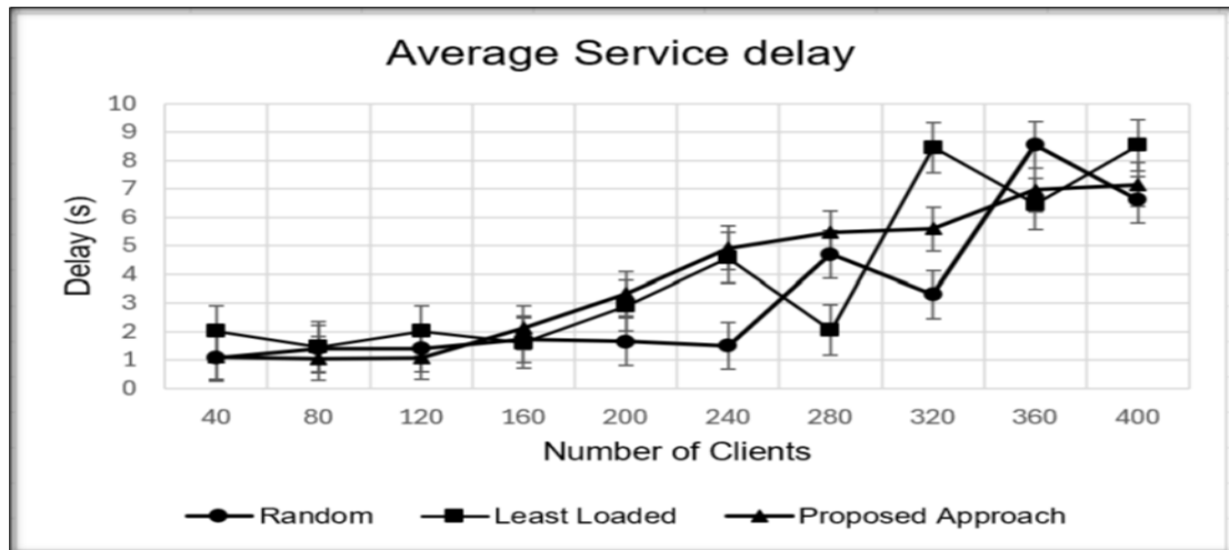
Figure 9.10 Average service delay for mobile users.
